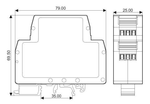
Can be installed on standard DIN35 rails
